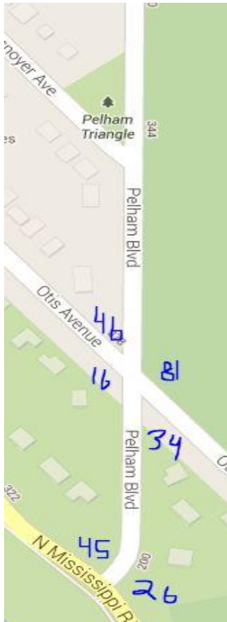
Figure 8: Curb Radii in feet, “River Road” and Otis intersections on Pelham Boulevard
